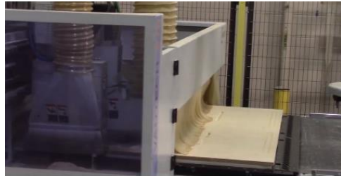
Correct material is selected and loaded, then parts are cut by our CNC routers, automatically switching between tools for desired finished appearance.
