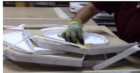
Parts are now hand trimmed to remove excess vinyl, placed with the order, and sent to packaging.
