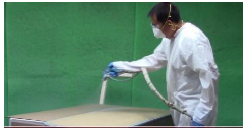
After parts are cleaned of debris, they are moved to the glue department. Surfaces that require vinyl are sprayed evenly and thoroughly.
