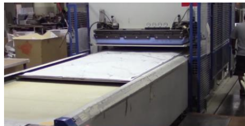
The parts are now sent into the press, where heat and pressure will form and adhere the vinyl to the substrate.
